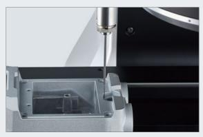
Even narrow locations are detected and measured automatically
