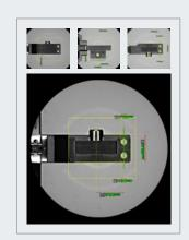
Measurement of multiple surfaces with a single setting
