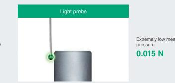
Since measuring pressure is extremely low, detection is possible without affecting the part
